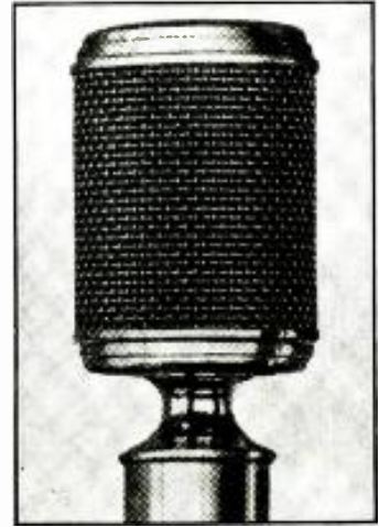
Above, left, Fig. 939B; directly above, Fig. 939A. Diaphragm-type crystal mike.
