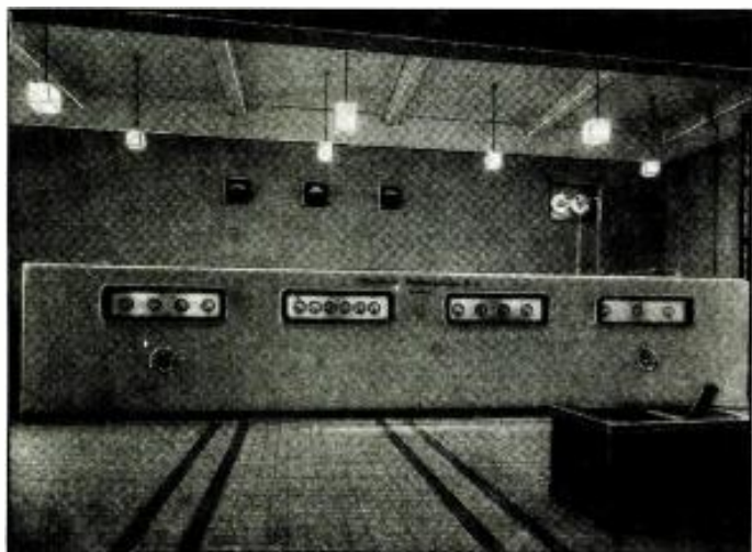
At left and right are shown two views of the Budapest broadcast station. The transmitter panel (left) is unique with its modernistic simplicity. The entire transmitter is controlled from the master monitoring desk in the right foreground. The antenna (right) is a half-wave radiator.
