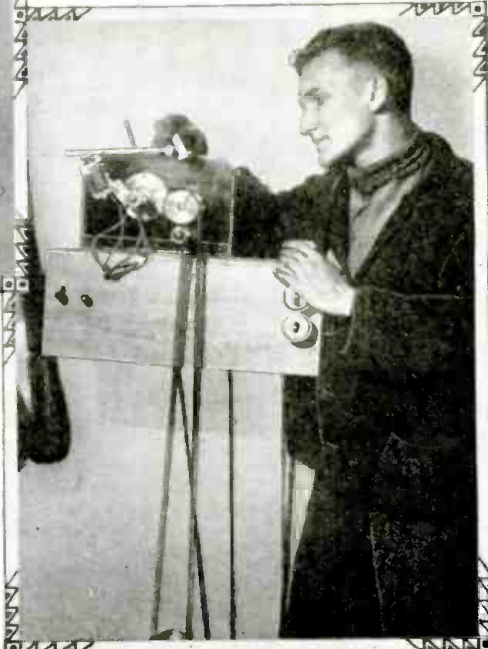
NEWEST TYPE KERR CELL. This was developed for television work by W. H. Peck. It is used to modulate the light beam; the bulb is almost entirely liquid-filled.
