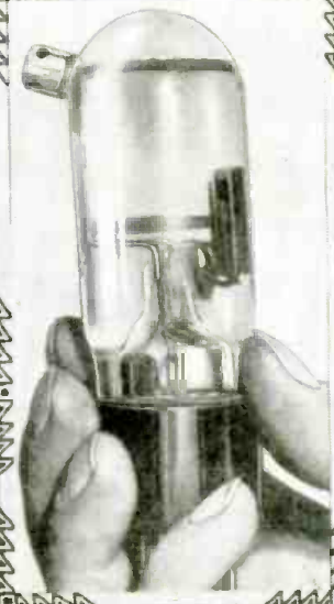
NEWEST TYPE KERR CELL. This was developed for television work by W. H. Peck. It is used to modulate the light beam; the bulb is almost entirely liquid-filled.
