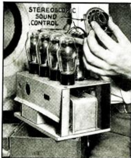
The single stereoscopic control knob on S. W. Coombs' portable P.A. amplifier.
